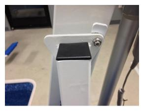
4. Tighten nut until snug against the bushing. Do not over tighten. 5. Locate the seat stabilizer bar, and raise it up and behind the triangle so that the bar is situated in between the triangle, and the main beam. 6. Insert the bolt that is pre-attached, ensuring that the 3 nylon washers are spaced in between the nut, the triangle and bar, and the bolt head. Tighten the nut until snug, but do not over tighten. 7 & 8. Finished Seat tube assembly.
