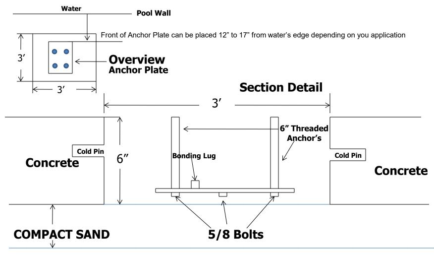
Optimal placement of the anchor system is 13" from the front of the anchor plate to water's edge. Attach copper wire to the bonding lug and then to your bonding grid
