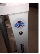
1. Insert the seat tube into the upper hole on the lift, ensuring the tube is inserted into the side with the protruding tube as shown above. 2. The seat tube will have to be cranked in a clockwise direction to thread thru the brass bushings. 3. Keep cranking until the threads protrude from the back side of the lift, and the triangle is butted up against the bushing.
